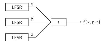
Boolean functions with large nonlinearity are difficult to approximate by linear functions and so provide resistance against linear cryptanalysis.
