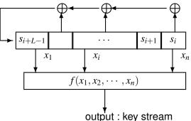
• A Boolean function takes as inputs several bits of a single LFSR to produce the key stream : a filtering (Boolean) function *f*
